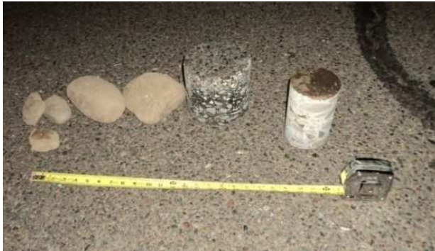
Picture 5 – AC and PCCP Cores Obtained at C9. Oversized rock (cobbles) were encountered in the lower portion of the ABC. The top of the PCCP included a roughly 1/4-inch thick layer of AC.
