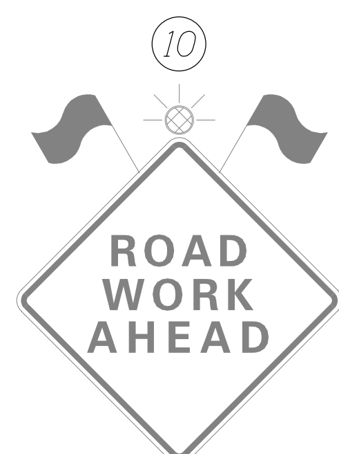
Existing W20-1 To be Maintained
