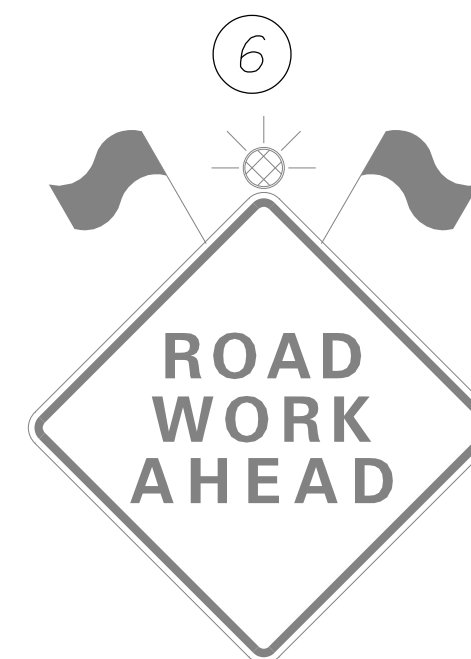
Existing W20-1 To be Maintained
