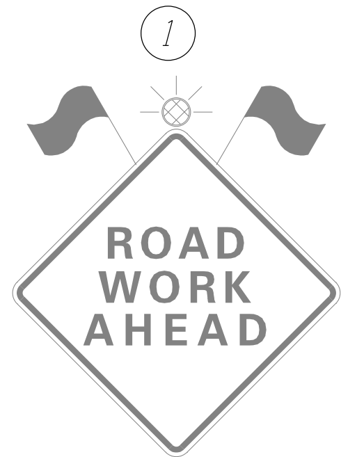
Existing W20-1 To be Maintained
