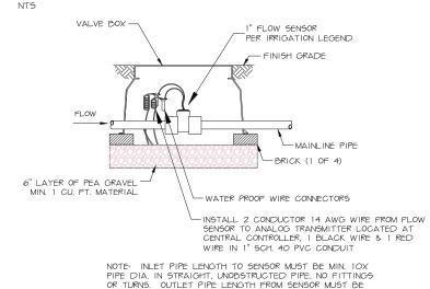
MIN, 5X PIPE DIA, IN STRAIGHT, UNOBSTRUCTED RUN OF
