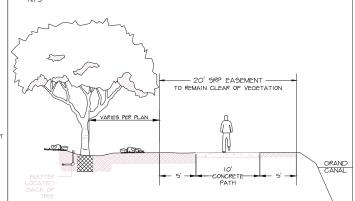
SRP MAINTENANCE EASEMENT AND PATHS REQUIRE VEGETATION CLEAR TO A HEIGHT OF 10 FEET. MATURE TREE CANOPY CAN NOT BE WITHIN SRP MAINTENANCE EASEMENT.
