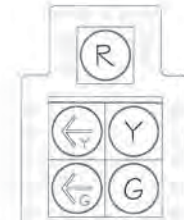
Type "Q2" with Plumbizer 5 Section 12" Signal Head Mounted on Signal Mast arm
